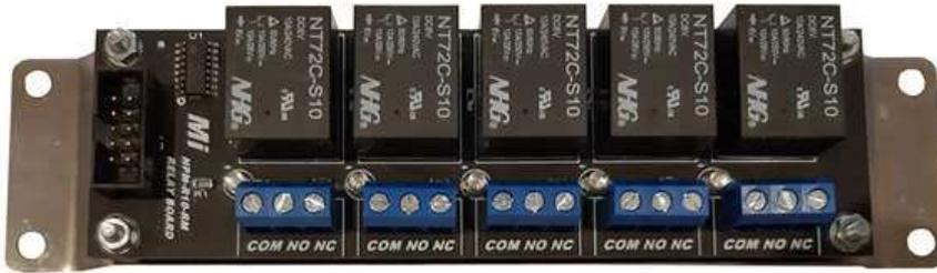
The 5 Relay expansion board connects to the Solar Monitor via a 10way ribbon cable supplied with the relay board, Relay's is rated at 10Amps 220Vac.
